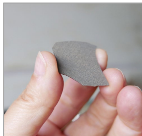
High-purity electrolytic manganese metal (HPEMM >99.9% purity)
